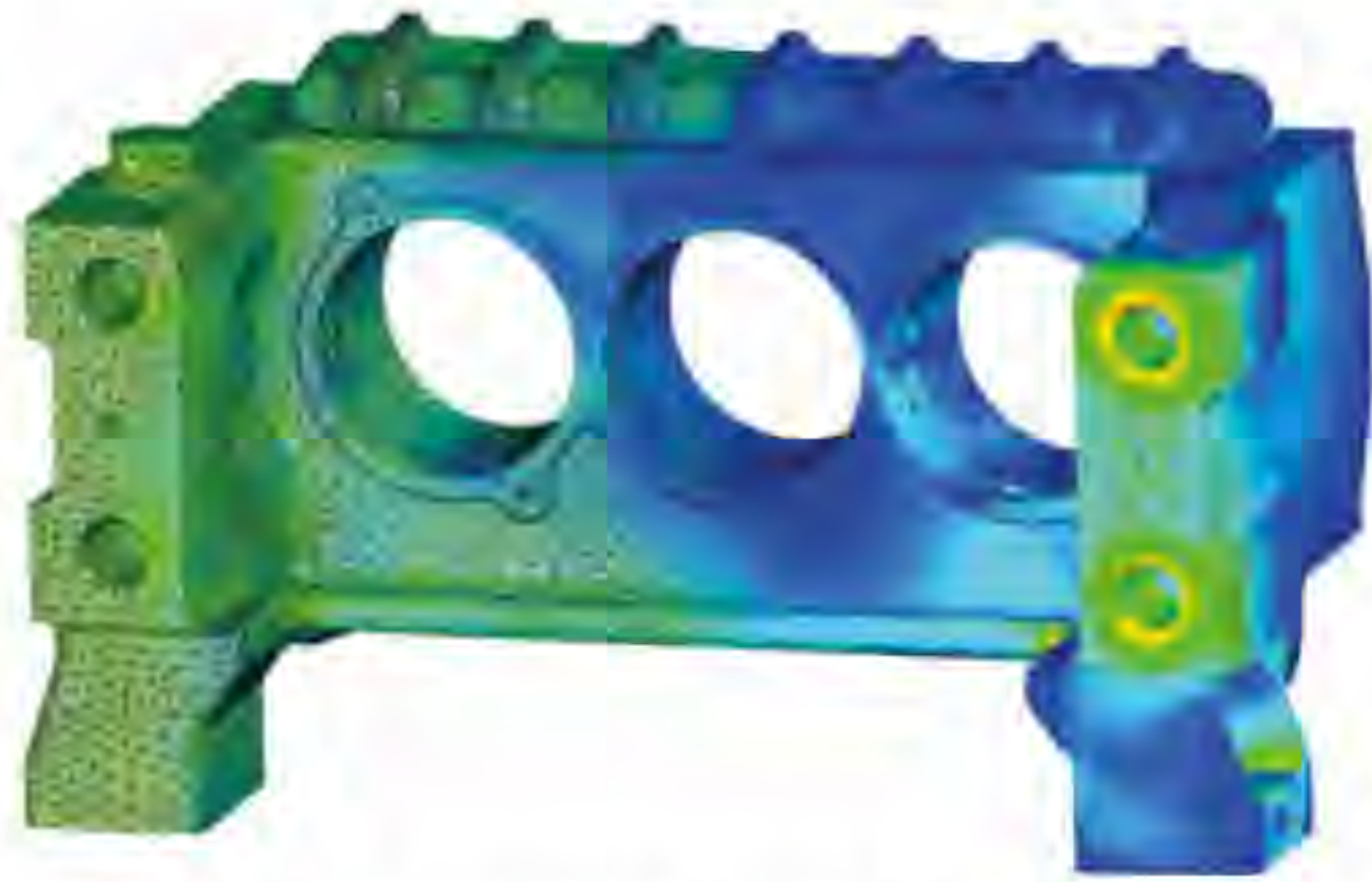
Modern simulation tools such as FEM and CFD support the design process at Wepuko PAHNKE.
