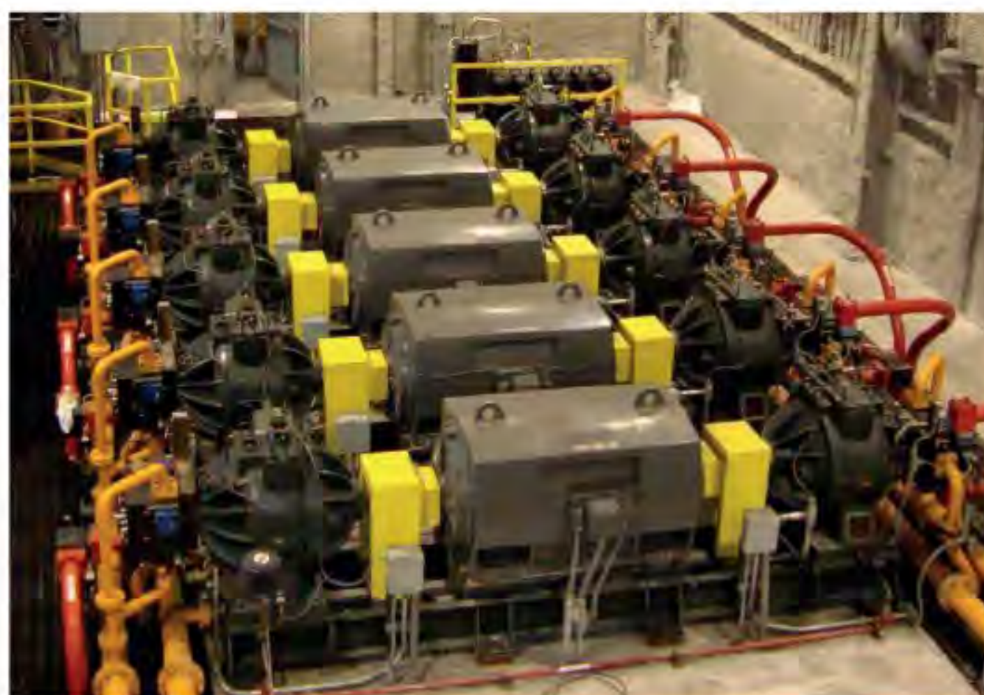
10-RX-pump PMSD drive for a 53 MN open-die forging press at Union Electric (USA).
