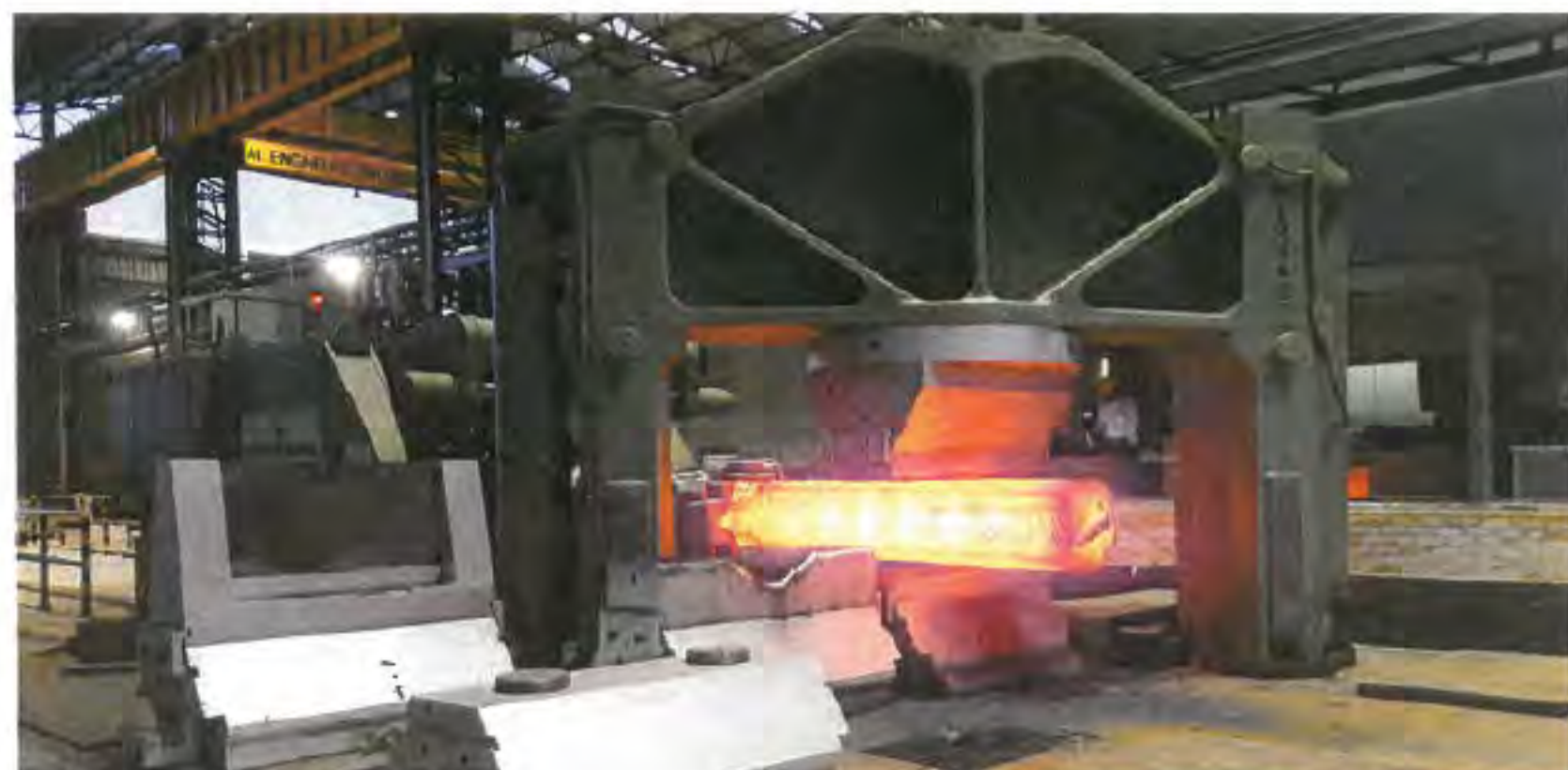
2017: A 31,5-38 MN pull-down open die forging press from PAHNKE at CHW Forge in India. The press features a PMSD drive with 6 RX pumps.
