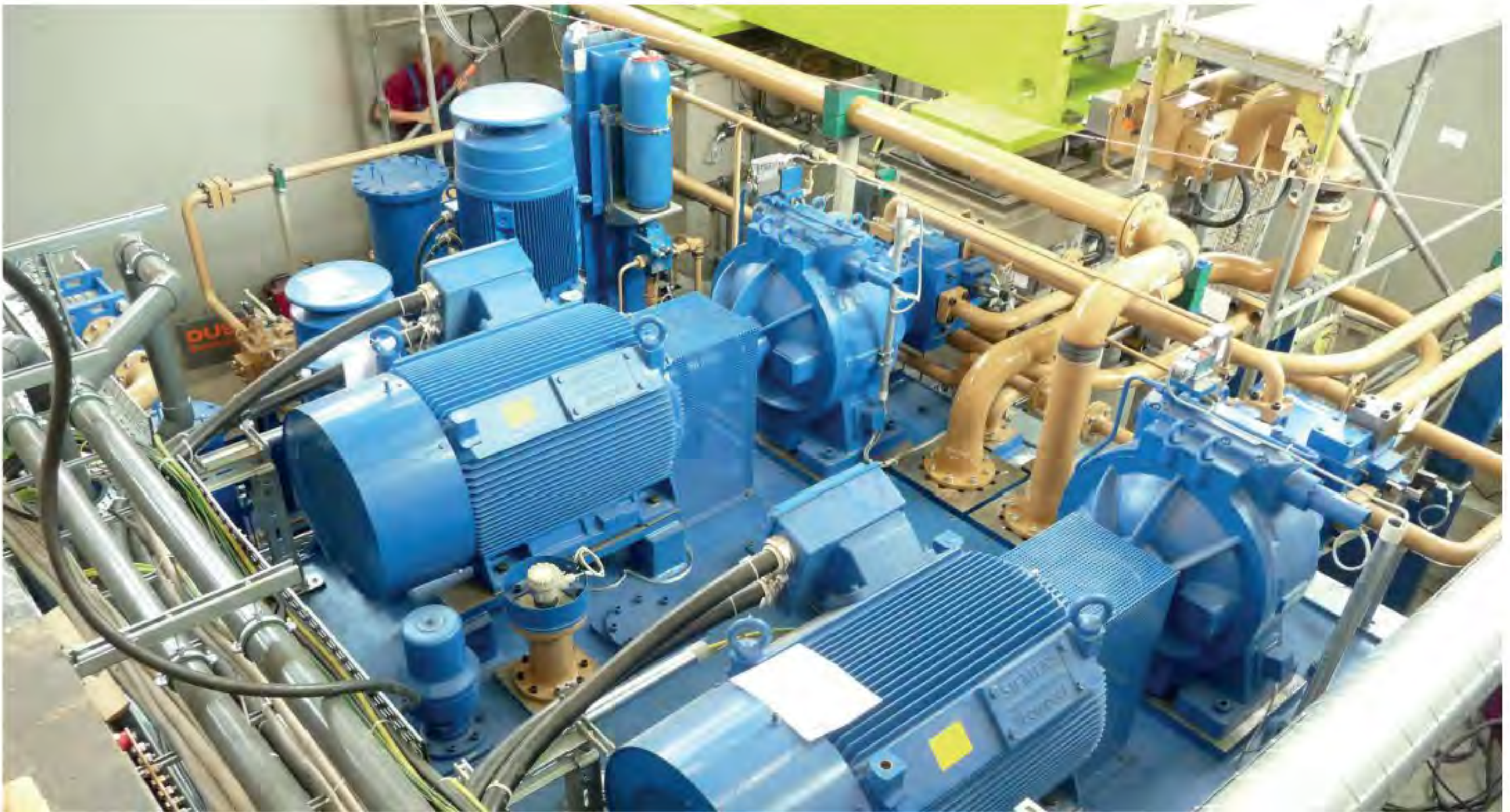
2-pump PMSD drive for the special press at the Freiberg University of Technology prior to commissioning
