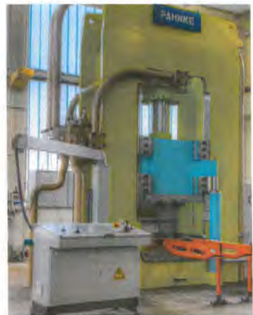
This particularly versatile 10 MN multi-function press is used at the Technische Universität Freiberg.
