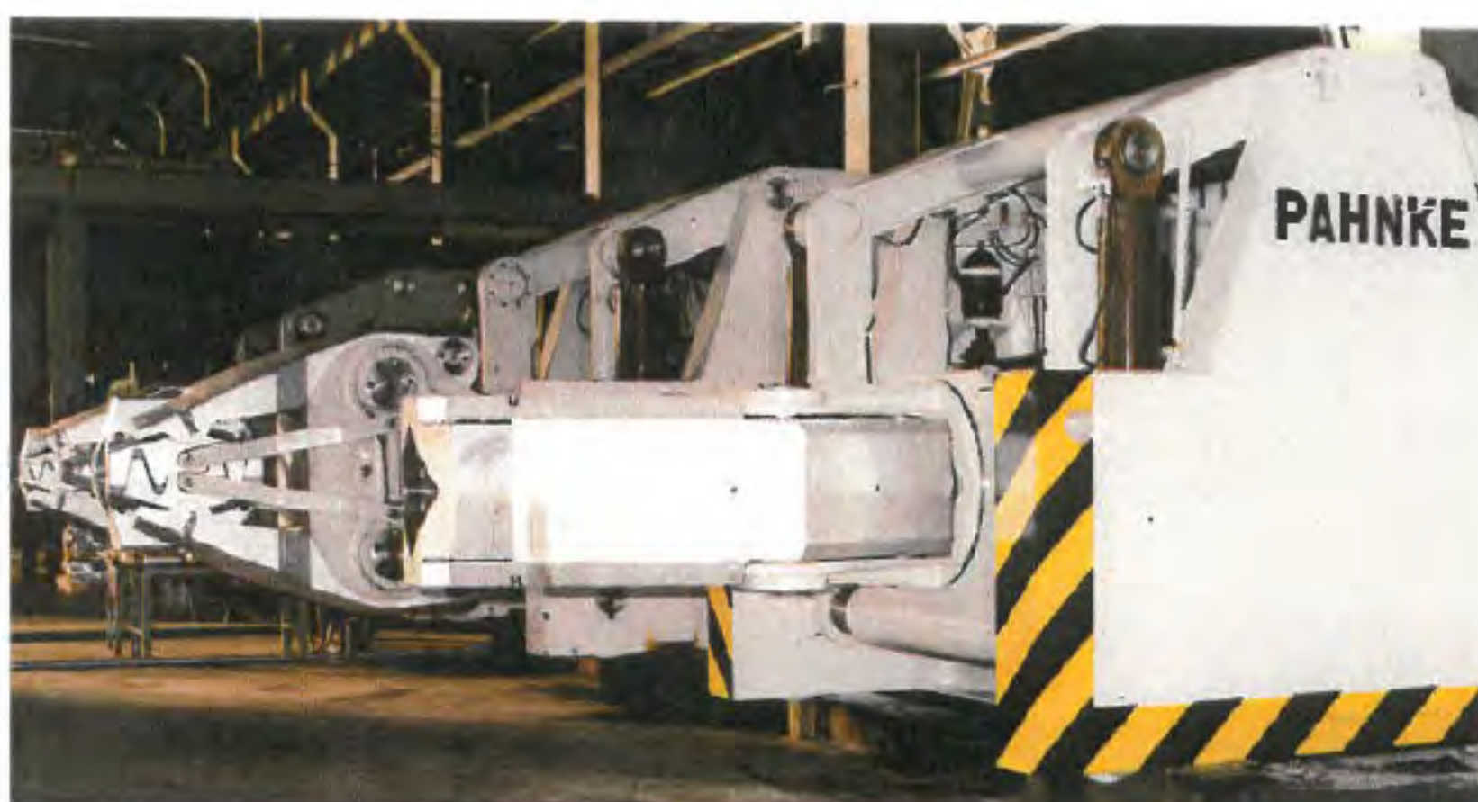
Wepuko PAHNKE forging manipulators enable the fast and precise positioning of heavy workpieces.
