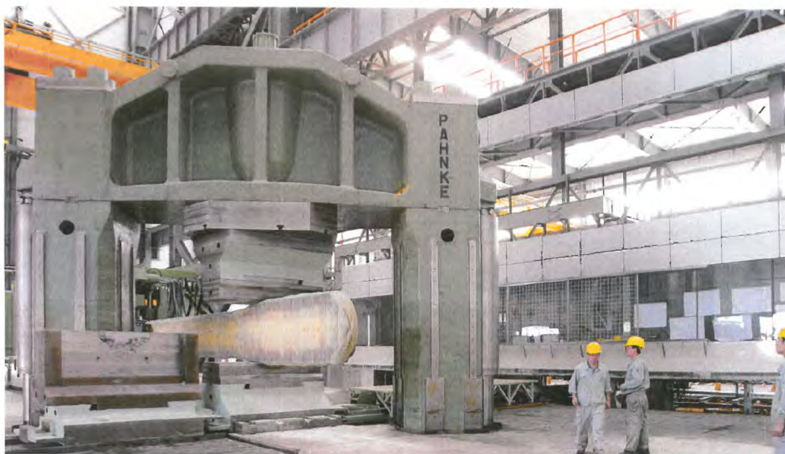
Forging of titanium and super alloys is very demanding. Baoti in China uses the world's most powerful and fastest open die forging press in the titanium industry made by PAHNKE (80/100 MN press force, two columns, pull-down design). It's PMSD drive, highly intelligent control systems and sophisticated design secure Baoti's leading position.
