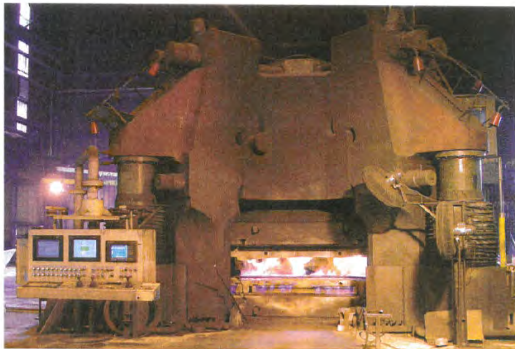
This high-performance closed die press with a press force of 300/350 MN is in use at Weber Metals, Inc., in the United States.
