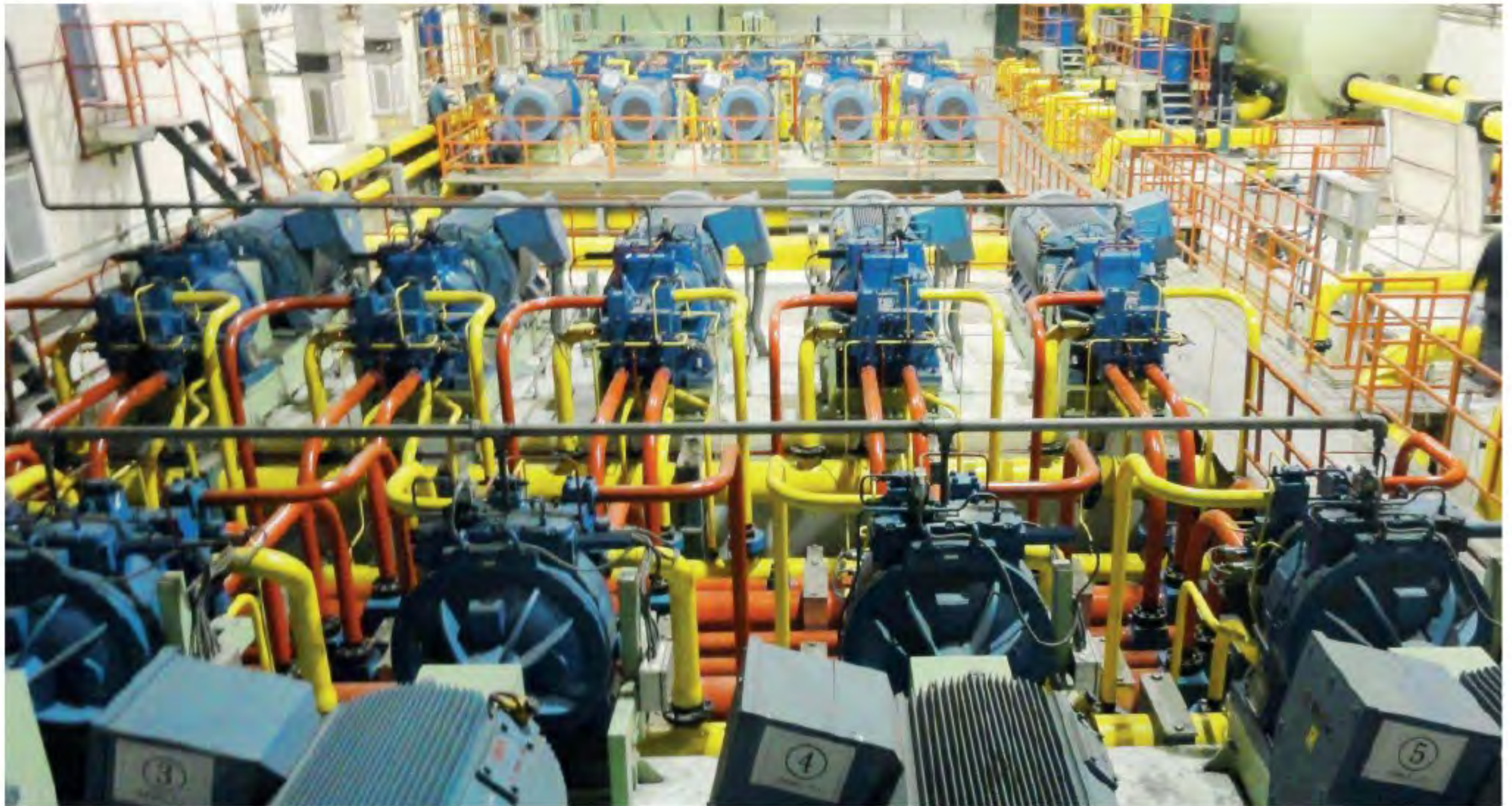
20-pump PMSD drive (RX 500) for a modern 185 MN press from PAHNKE.
