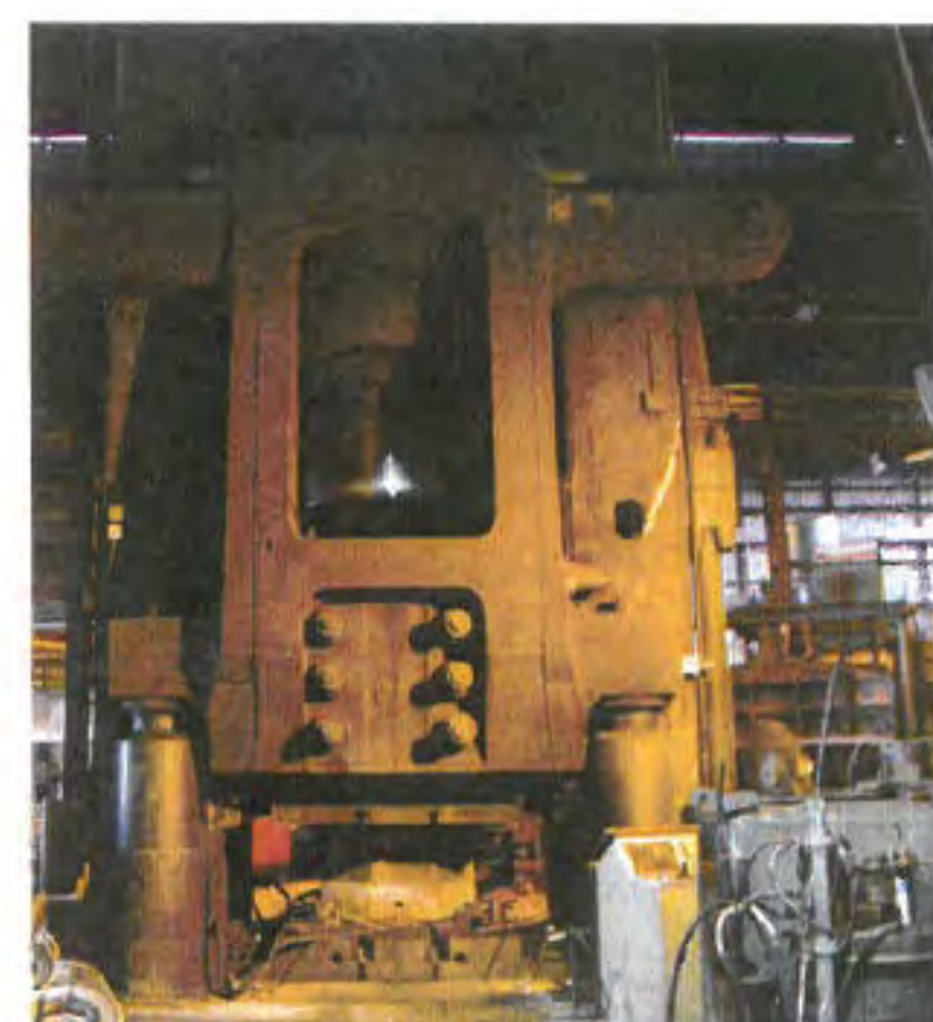
This closed die 110 MN press is located at Weber Metals, Inc., in the United States.
