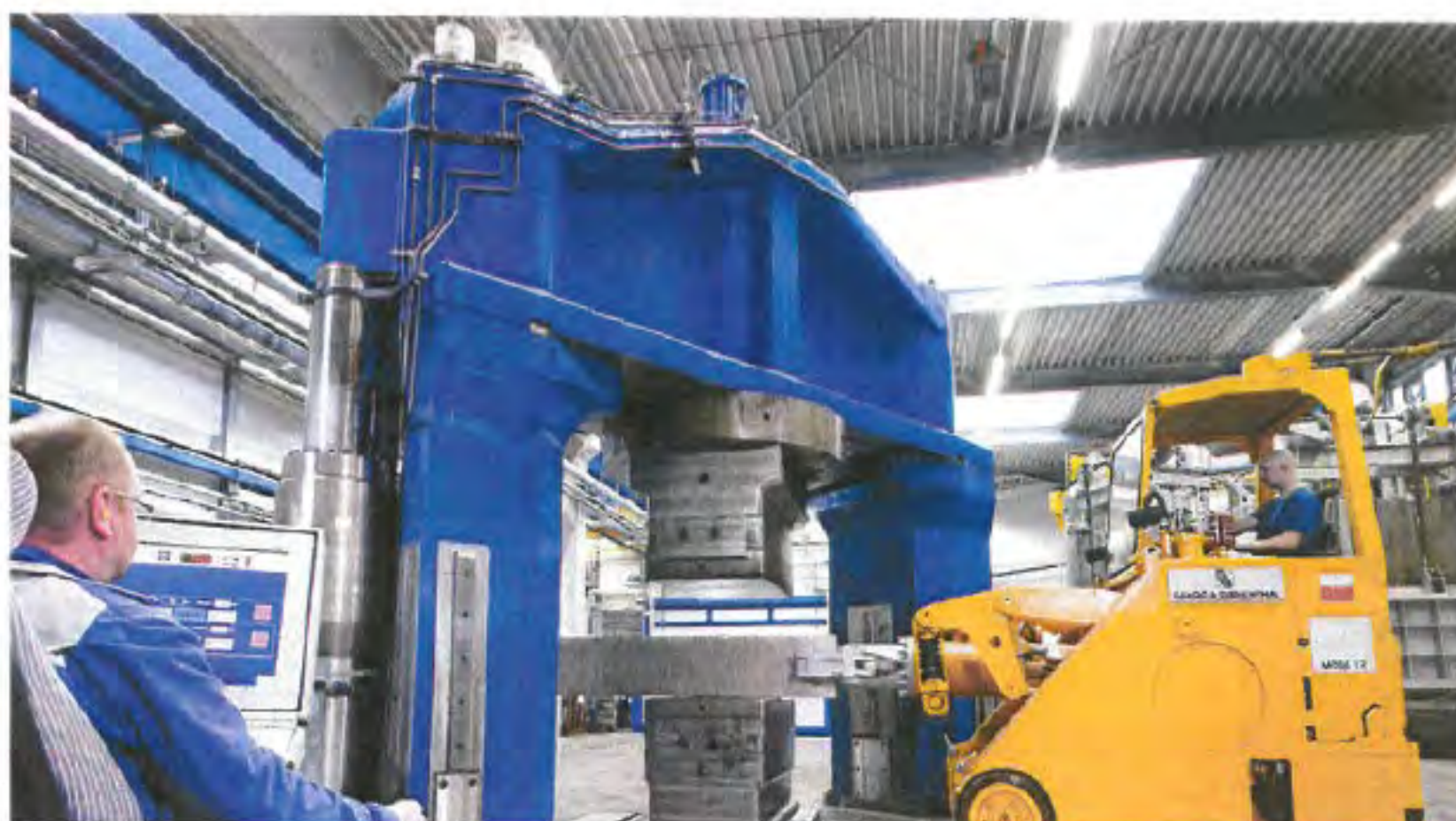
The new, quick-action open die forging press at OTTO FUCHS KG, Meinerzhagen, Germany, mainly forges products for aerospace applications and plant construction. The press force amounts to 30/36 MN. The press uses the PAHNKE Modified Sinusoidal Direct drive (PMSD drive) and was constructed in a two-column design.
