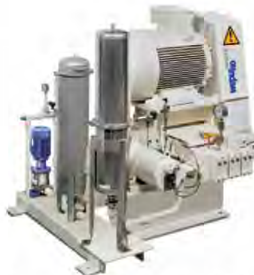
Compact version of the pump unit DP 405 for the cooling of tools including booster pump and filters (suction side) and resonator for pressure pulsation dampening (pressure side).
