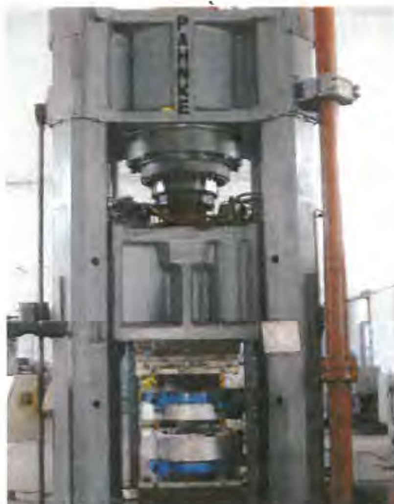
An example from the portfolio of Wepuko PAHNKE is this 20 MN multi-function press with force levels of 15 and 6 MN with installed isothermal forging tools.
