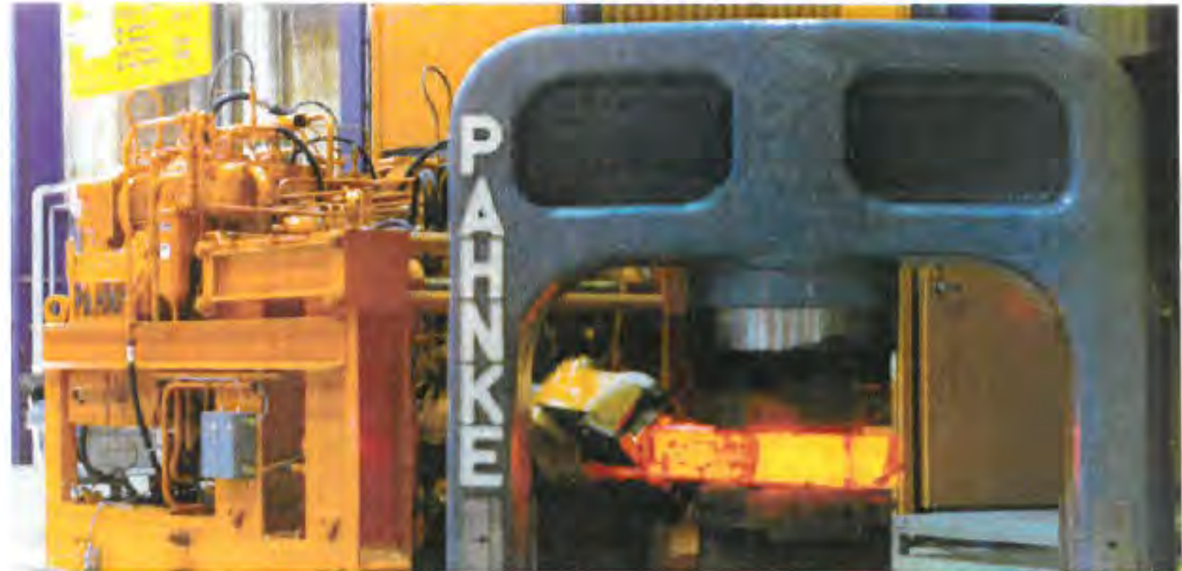
1976: The first PAHNKE press with the first PAHNKE Modified Sinusoidal Direct drive (PMSD drive). The press force of the pull-down open die press is 5 MN.
