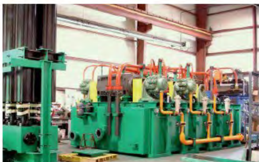
8-RF-pump drive for the 10,000-tonne closed-die forging press at Standard Steel (USA)
