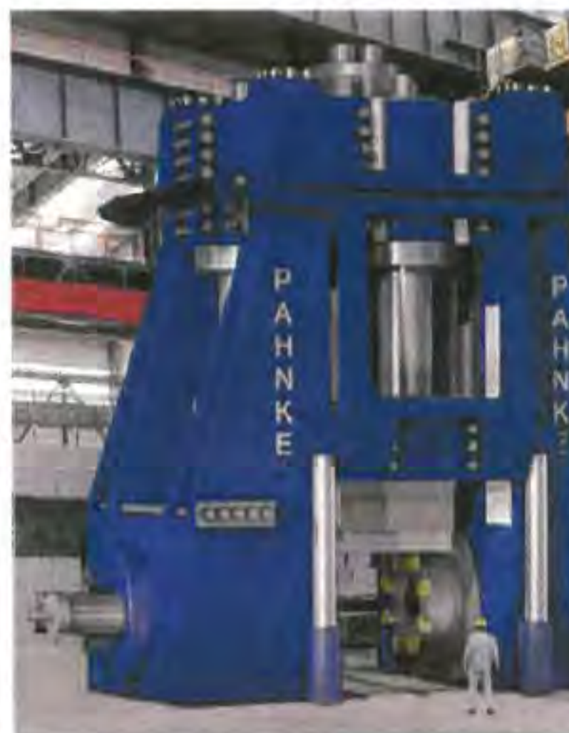
This 200 MN multi-cylinder press manufactures forged valve bodies for use in the oil & gas industry.
