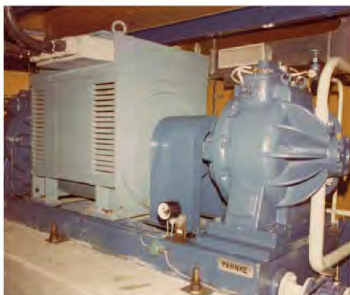
The first PMSD drive (1976) for a 5 MN forging press
