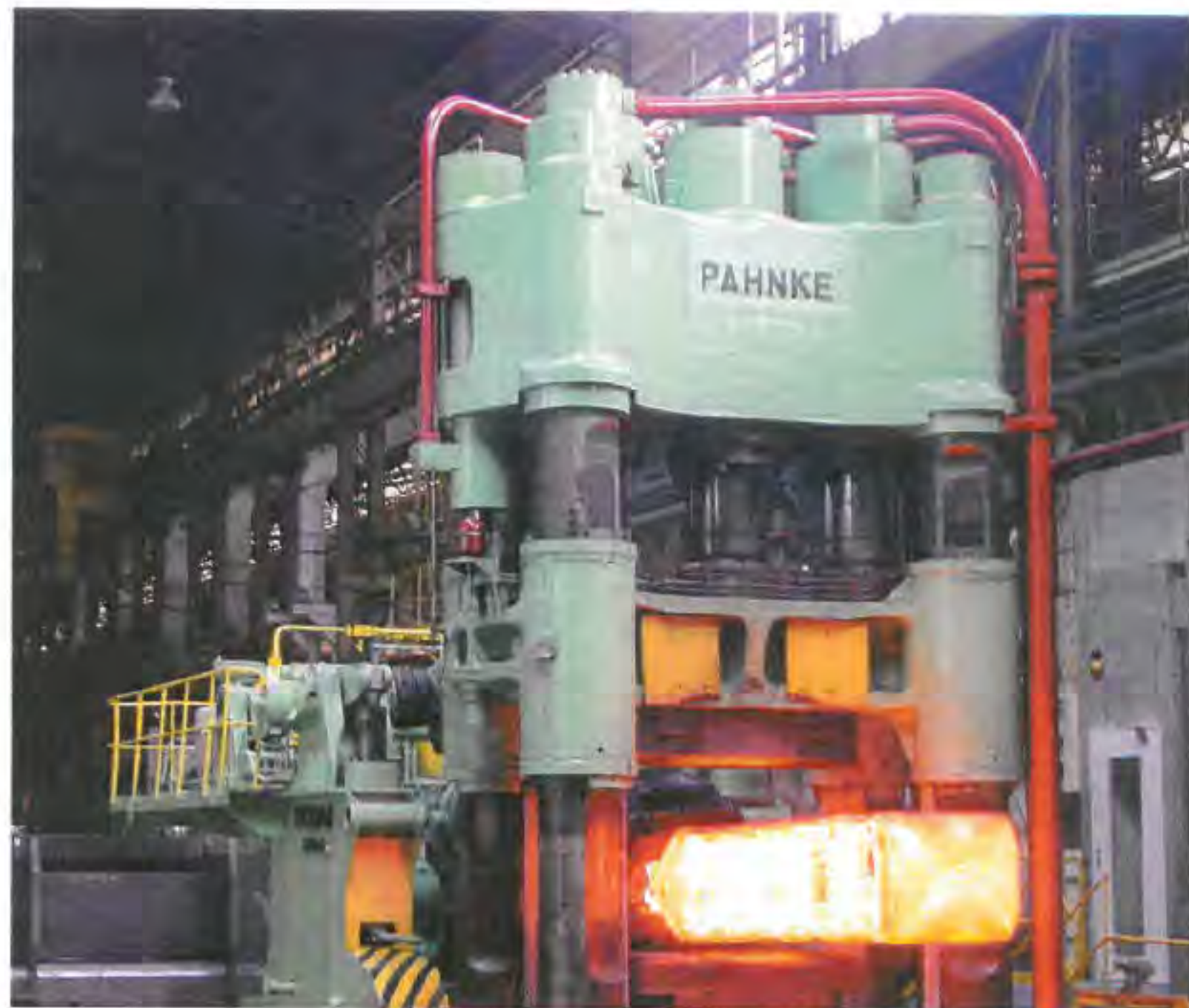
This modernized open die press with three cylinders has the following technical data: Press force levels 18 MN (two-cylinder operation) and 27 MN (three-cylinder operation), compressive force: 30 MN, drive 8 x RF 650 radial piston pumps with valve control system.
