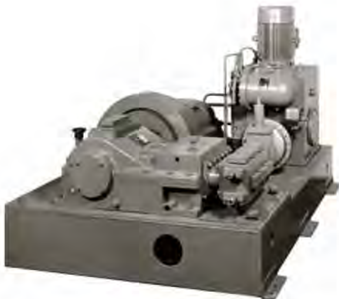
Horizontal triplex plunger pump from the year 1955.
