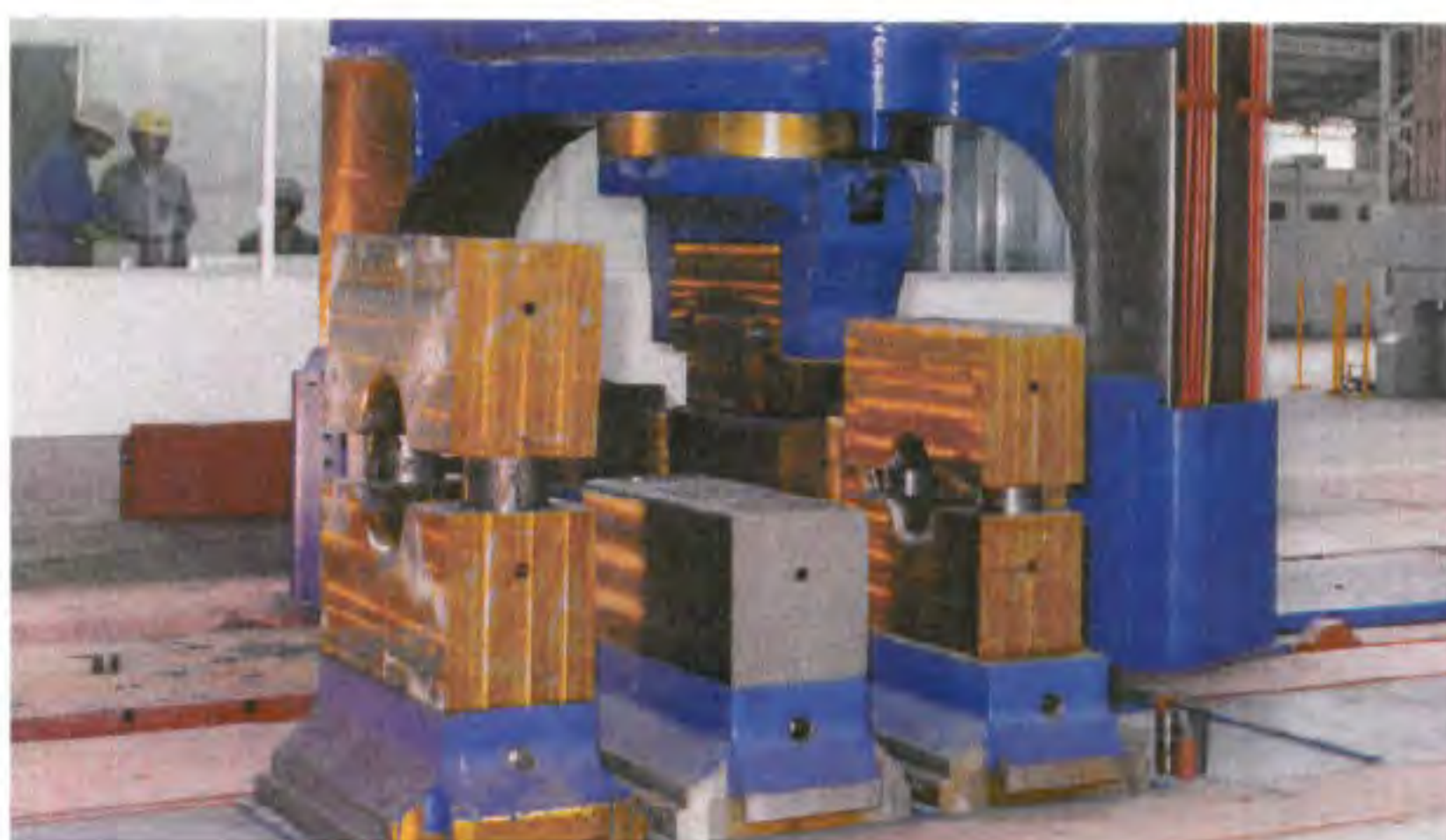
Quick-changing tool system of an open die forging press.
